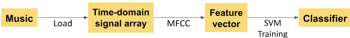
Figure 3. The high-level workflow of the instrument identification algorithm
